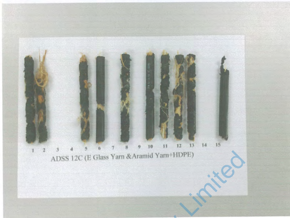
Figure 1. Damages from rat gnawing activity on Cable ADSS 12C (E Glass Yarn & Aramid Yarn + HDPE) on Day14. Numerical numbers indicate rat identification.
