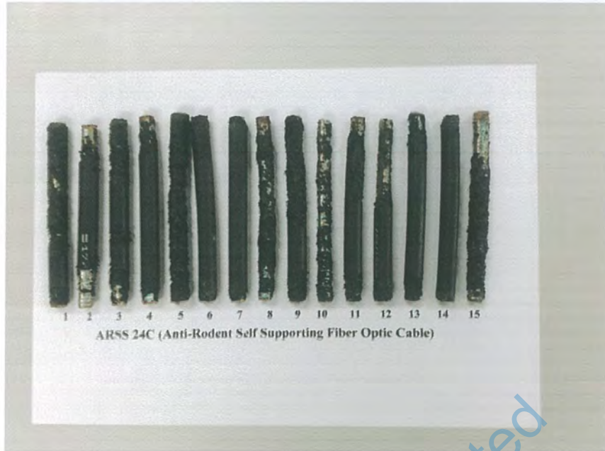
Figure 1. Damages from rat gnawing activity on ARSS 24C (Anti-Rodent Self Supporting Fiber Optic Cable) on Day14. Numerical numbers indicate rat identification.
